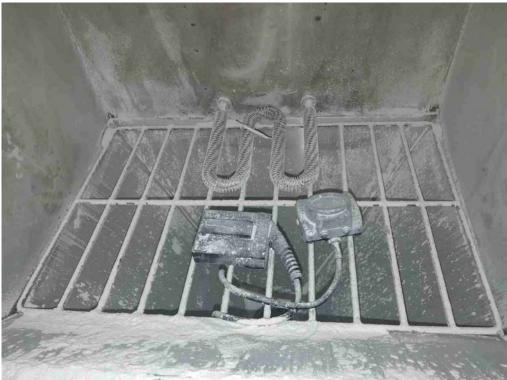
Photo 2: After dust test view (IP6X test)
