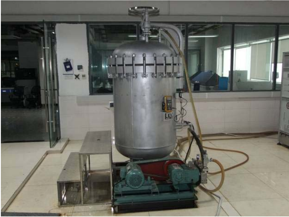
Photo 4: Water test view (IPX8 test)
